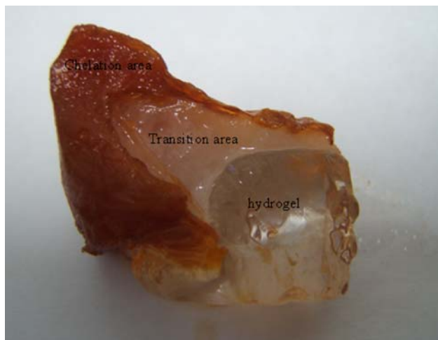
Fig. 4 Profile morphology of chelate PAC/PEG IPN hydrogel
